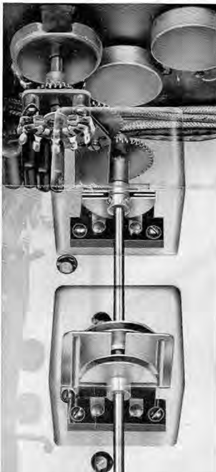
Section of Selectivity-Fidelity Control Mechanism.
