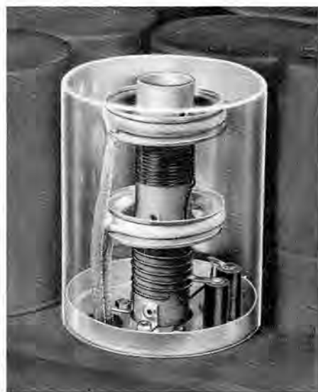
The Scott Supershield Antenna Coupling Unit Used on Foreign Short Wave Bands.
